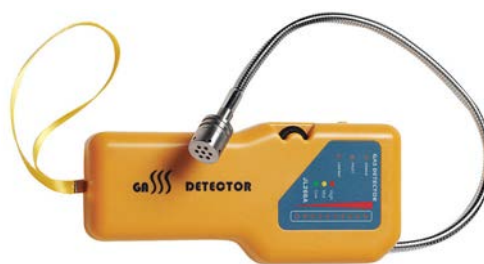
Figure 31. Typical hand-held portable methane detector. Photo from Gladstein, Neandross & Associates, NREL 44691
