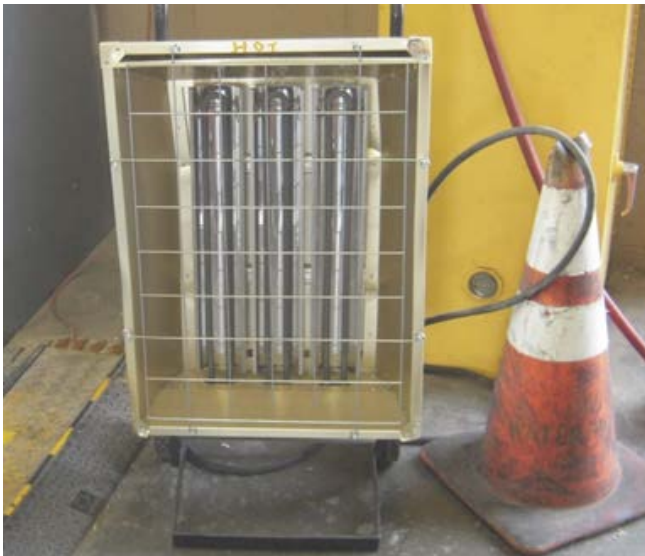
Figure 20. Floor-mounted portable propane heater should be eliminated. Photo from Gladstein, Neandross & Associates, NREL 44905
